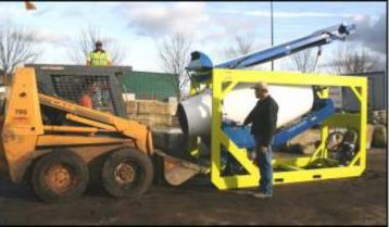
The loading, mixing and dispensing of the concrete materials are all completed inside of the box, reducing the amount of equipment needed at the job-site. The mixing process is simplified by the use of an on-board material loading conveyor. Just load the top-mounted conveyor with the sand and gravel and it will flow into the drum for mixing. The drum spins in both directions for mixing or
